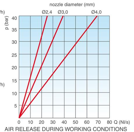
The air flow charts were created in Kg/s from laboratory tests and numerical analysis, without the screen, then converted in Nm³/h using a safety factor.
